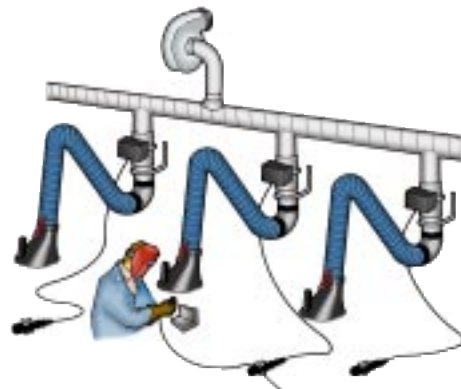
If you connect several extractor arms to a central system, you should install automatic dampers to maximize fan power.
